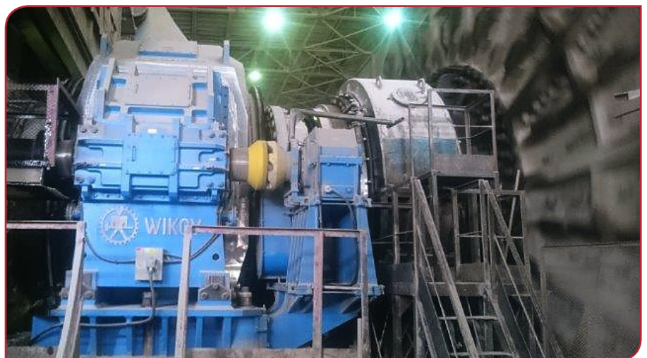
Below: The gearbox is 8m long, 5m high and 2.5m wide. Since it started operation, Spassk-Cement confirms that the drive has run without problems for 1776hr. It has ground an average 264t/hr of cement. This means that it has ground over 468,864t of cement.
